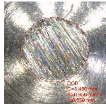
Fig. 10: Wear marks on hardened C45E steel with nACVlc coating after 1000 revolutions
