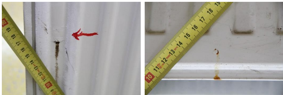
Fig. 1: Delivered radiators and location of wall perforation and leakage. Paint blistering at the site of the leak.
