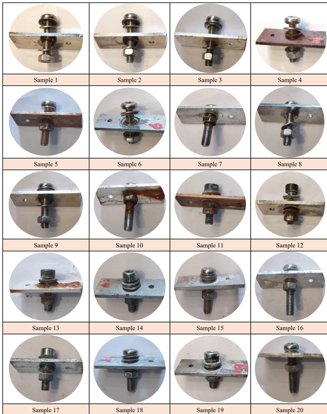
Fig. 10: The appearance of unscrewed samples 1-20 after 96-hour test in the salt chamber
