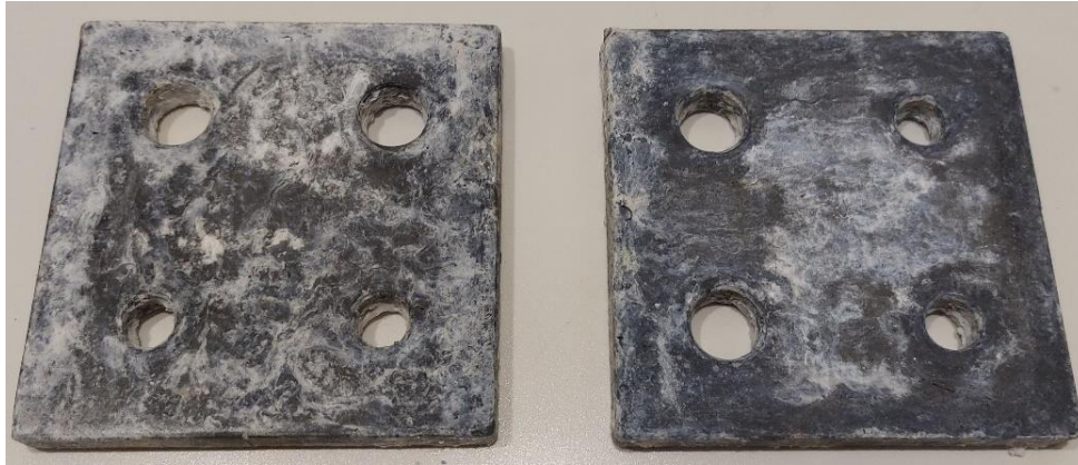
Fig. 2: Metal zinc coating on a steel substrate after 720 hours of cyclic corrosion aging test on corrosion protection system 1
