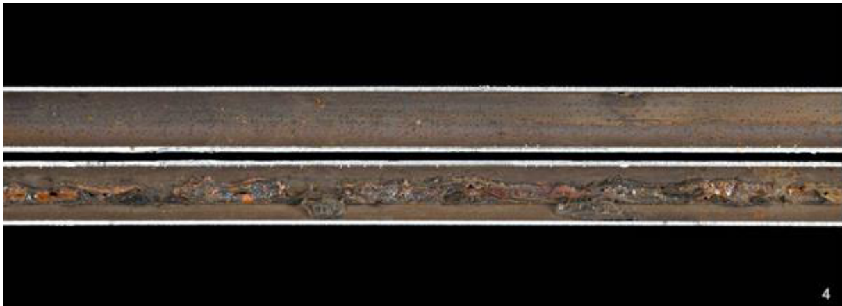
Fig. 4: Corrosion of heating pipes, damage from inside.
