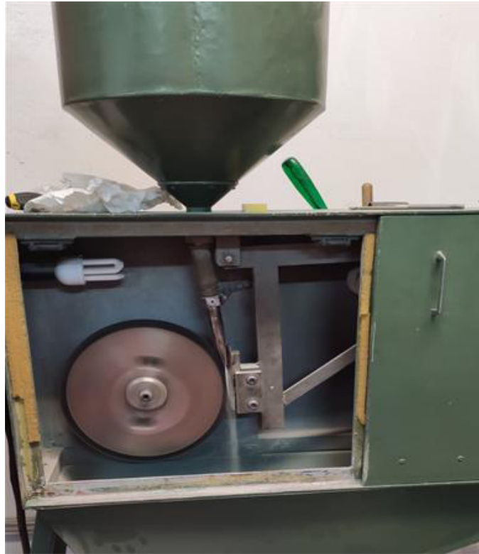
Fig 3: Device for testing resistance to abrasive wear using the "dry sand-rubber wheel" method
