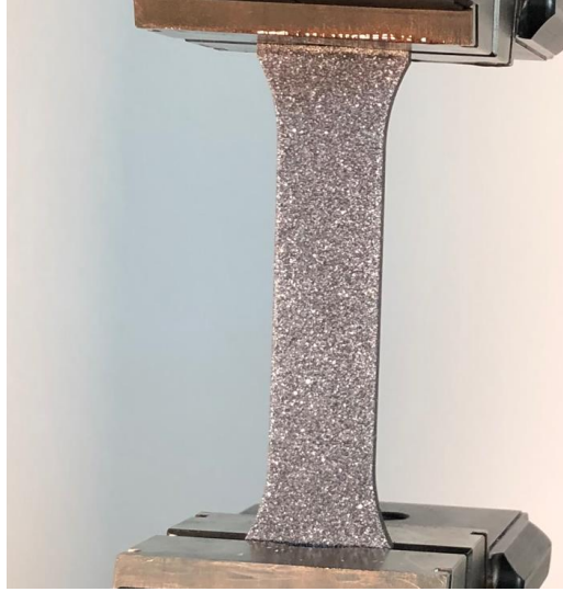
Fig. 2: Sample prepared for DIC experiment
