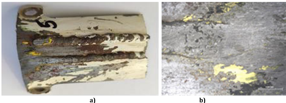
Fig. 4: Partially worn helicopter skid shoe: a) the entire shid shoe, b) the surface of the welded layer
