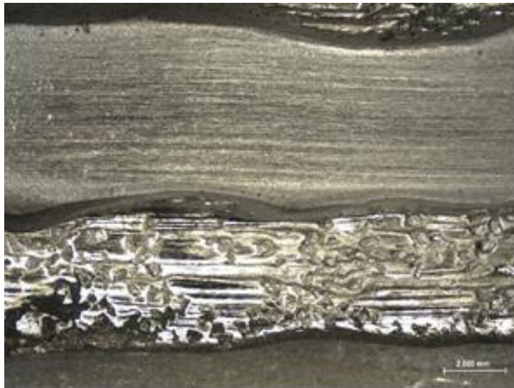
Fig. 7: Weld surface W1 after 5 min wear according to the "dry sand-rubber wheel" method
