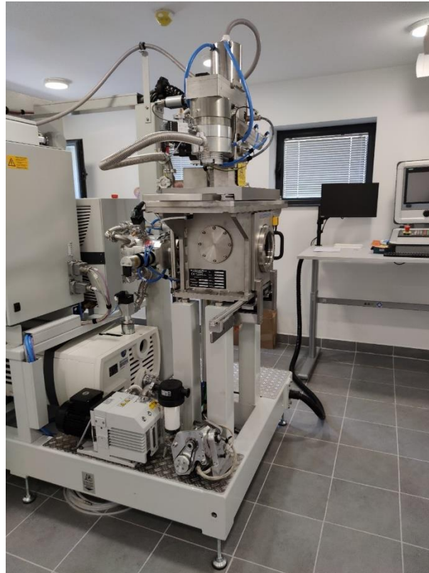
Fig. 1: An image of electron-beam treatment equipment at the Technical University of Gabrovo
