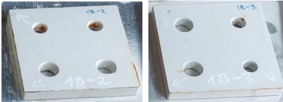
Fig. 6: Zinc rich organic coatings on steel substrate after 480 hours of cyclic corrosion aging test on corrosion protection system 8
