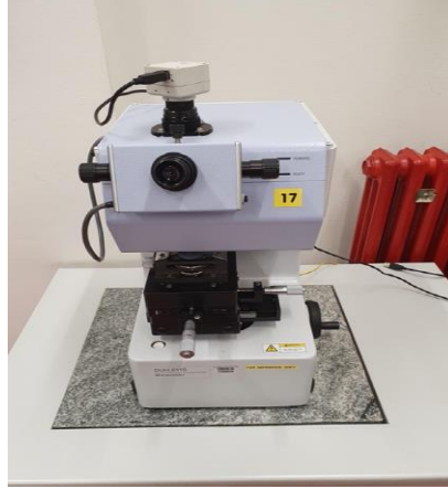
Fig. 5: DUH-211/211S nanohardness testing device
