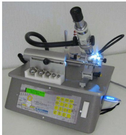
Fig. 2: Calotest thickness testing machine
