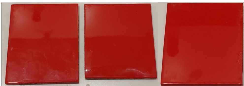
Fig. 5: Organic coatings on aluminium substrate after 1680 hours of cyclic corrosion aging test on corrosion protection systems 5 (left picture), 6 (middle picture) and 7 (right picture)
