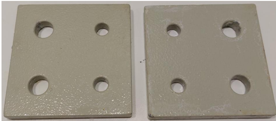
Fig. 3: Organic coatings (powder coating) on a zinc metal coating on a steel substrate after 1680 hours of cyclic corrosion aging test on corrosion protection system 2
