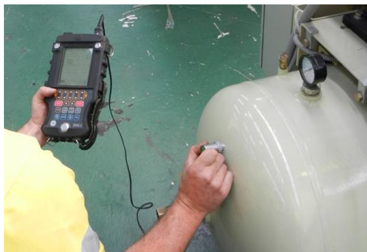
Fig. 2: Ultrasonic wall thickness measurement through the coating
