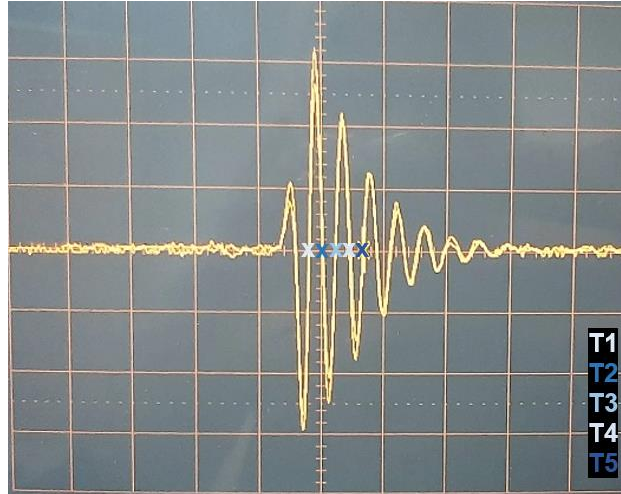
Fig. 4: Display of measurement points on two overlapped signals reflected from the back wall of the sample
