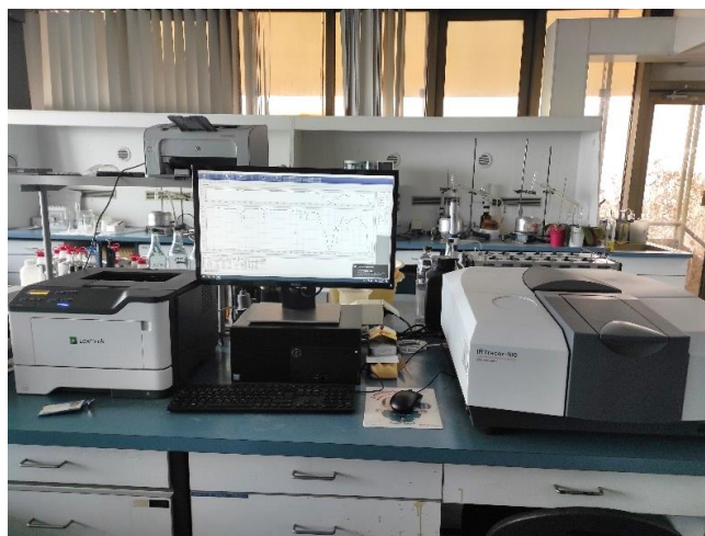
Fig. 3: FT-IR Spectrometer, IRTracer-100: SHIMADZU (Shimadzu Corporation)
