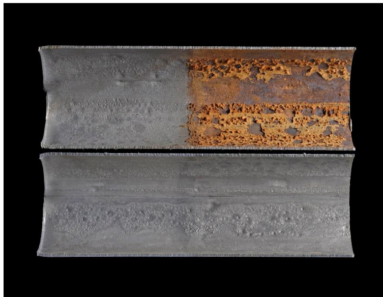
Fig. 2: Corrosion in a cooling circuit, grooving corrosion at bottom pipe half shell.
