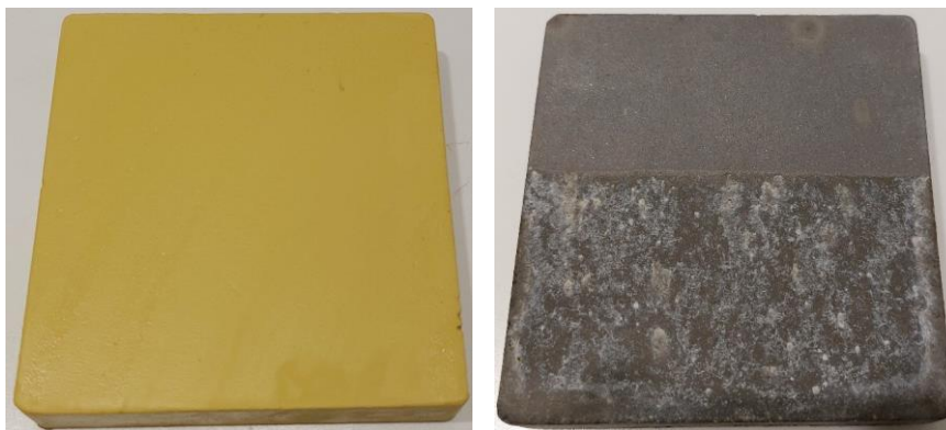
Fig. 4: Organic coatings on a zinc flake metal coating on an aluminium substrate after 1680 hours of cyclic corrosion aging test on corrosion protection system 3 (left picture) and corrosion protection system 4 (right picture)
