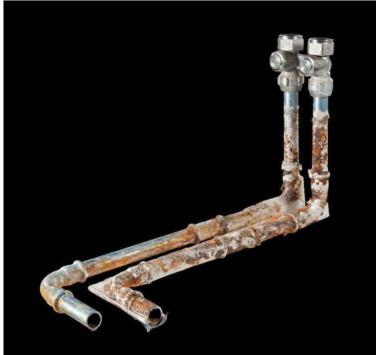
Fig. 3: Corrosion of heating pipes, damage from outside.
