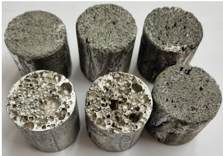
Fig. 1: Aluminium foam samples foamed with different foaming agents
