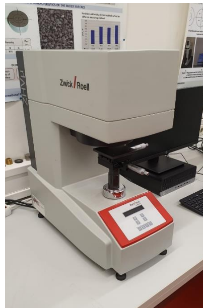
Figure 4. Zwick ZHV \mu hardness testing machine
